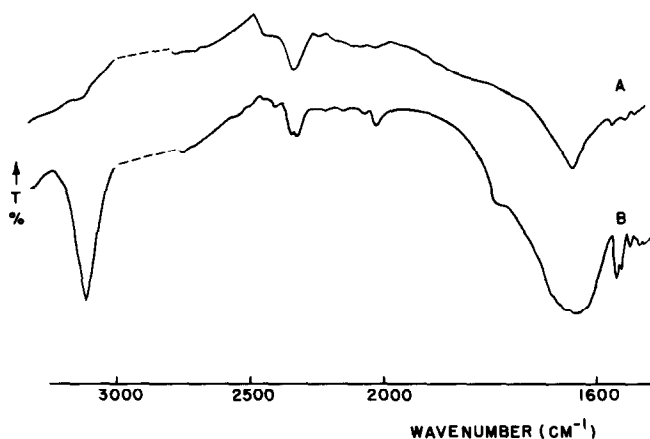
FIG. 2. Infrared spectra of CuY. (A) Evacuated at 200°C for 4 hr; (B) furfural adsorbed at room temperature.
